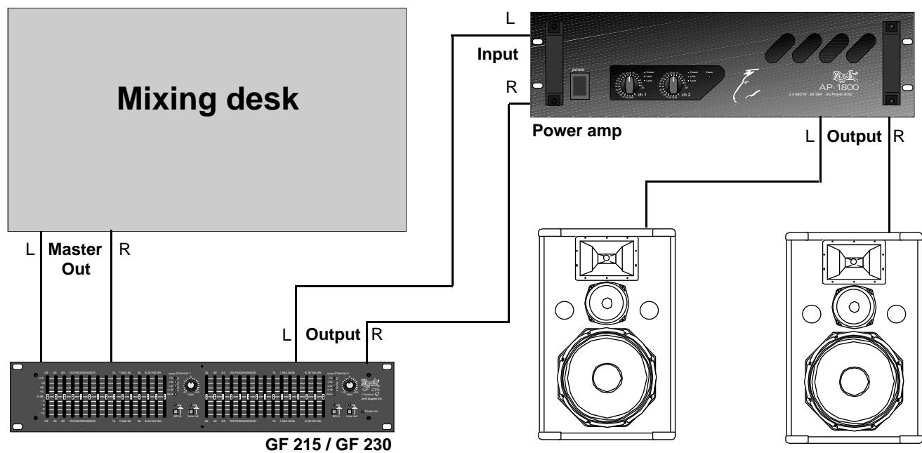
Connecting unbalanced devices to the GF equalizer is done easiest by using monaural phone jack instrument cables.
