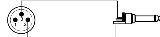
Connecting electric guitars / basses to the transmitter requires an electrical open pin 1. A special adapter cable is available as supply part **DSGK**.
